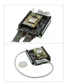
The USB-2COM-BB is a plug-in RS-232 cape designed for the developers and users of BeagleBone and BeagleBone Black. The USB-2COM-BB BeagleBone RS-232 cape provides two high-speed RS-232 serial interfaces, two high-efficient USB 2.0 ports and one Micro SD card reader. The two RS-232 serial ports are located to the side of the cape with two 90-degree 10-pin connectors.
