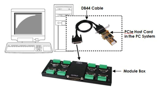
10. Up to 4 Modules can be daisy-chained to provide 32 ports. No other DIP switch or software settings required.
