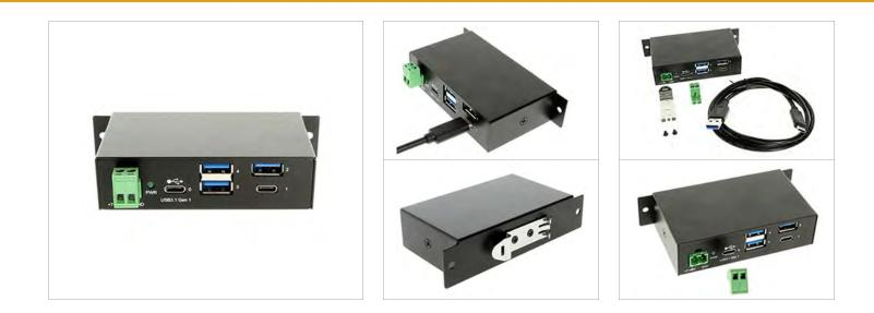
USB C hub provides 4 USB 3.1 Gen1 ports to include 3 USB-A ports and 1 USB C port. 1 Downstream and 1 upstream port use the reversible USB C connector. USB C hub is a Gen1 hub using USB 3.1 to support Super-Speed 5Gbps data transmission speeds and takes advantage of the reversible type-C port in both directions. This hub is self powered with a 2-pin terminal block connector to supply power input of +7 ~ 48V DC sold separately.
