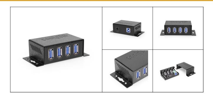
ESD and Surge protection over each individual USB 3.1 port. An industrial-grade USB 3.1 Mini 4 Port Hub that gives you up to 5Gbps of data transfer speed and a surface mount capability. Includes and 5V DC input jack for self-power option.
