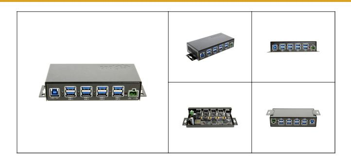
The unique design of this hub allows you to use seven (7) USB Type-A data ports and 1 (1) USB Type-A dedicated charging port. Its unique eighth (8th) port is a charge only port, no data, supporting 25W of power using QC2.0/3.0 quick charging technology and BC1.2 battery charging specifications.
