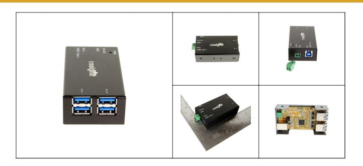
Built with industrial environments in mind, the USB 3.1 micro hub with 4 ports is a compact solution. Compliant with USB 3.1 specifications, the hub has data speed up to 5GBps. It includes a surface mounting kit but can be mounted on a DIN Rail.
