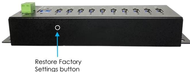
3. Use a paper clip or similar object to press and hold the Restore Factory Settings button, while still holding the button power on the hub.
